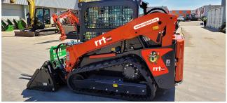
The Skidsteer machine is used to lift and load sand into the sand bagging machine, and transport pallets of sand bags.
