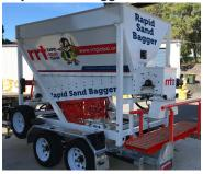
RRT's Rapid Sand Bagger can fill over 1,500 sand bags per hour, and is portable so can be deployed right across Australia.
