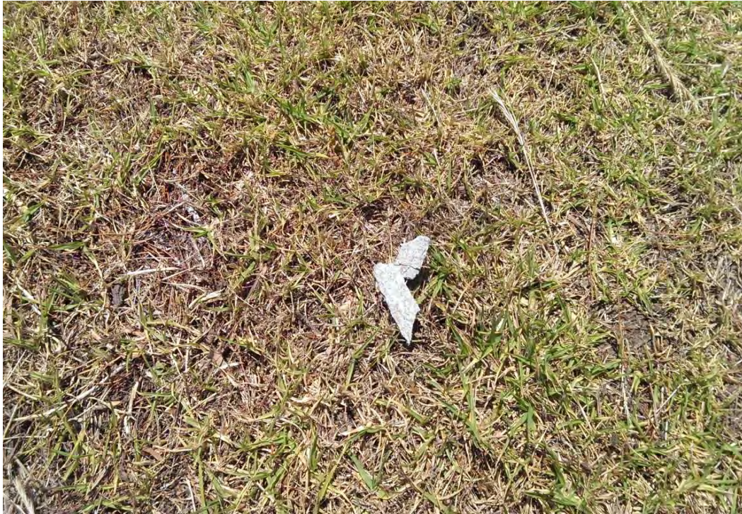
Photo 15 - damaged asbestos fragments adjacent to corrugated Asbestos sheet (AEC4)
