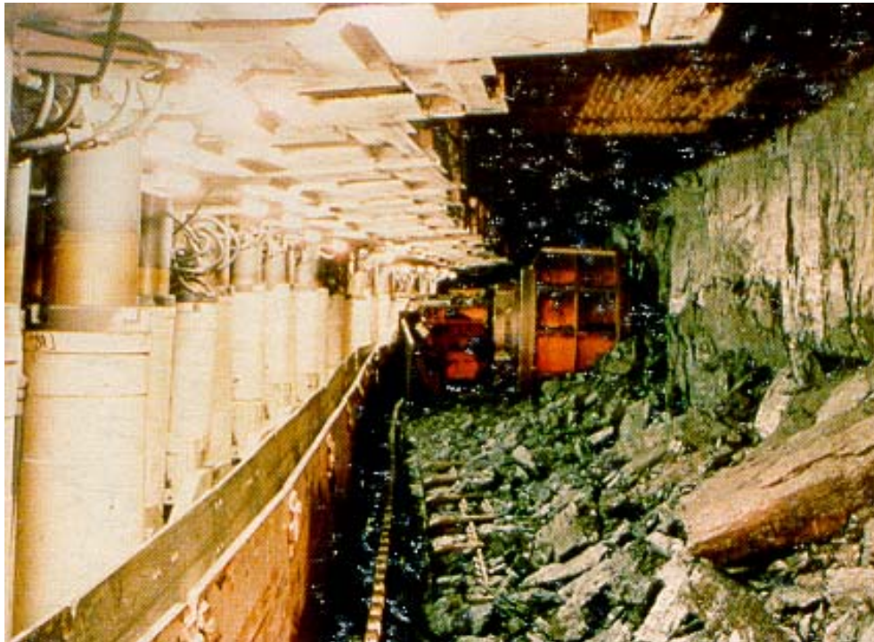
Figure C3 Typical Longwall Face Equipment
