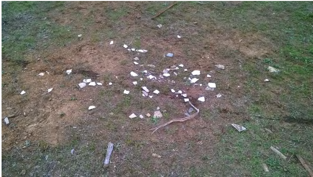
Photograph 13- ACM on the ground surface 10 m north of the former stockpiles. Photograph taken 9/7/18
