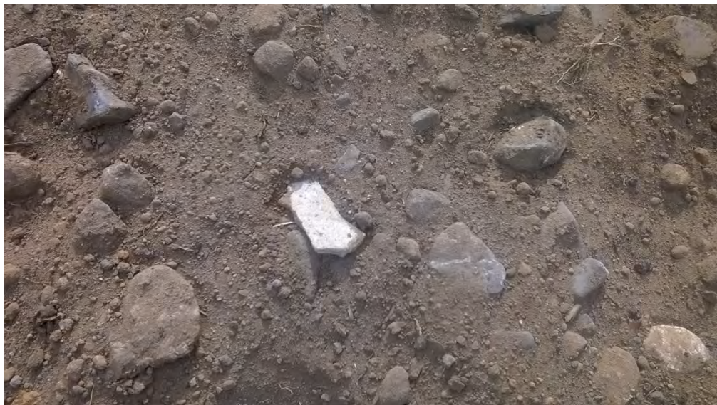
Photograph 11- Suspected ACM in the footprint of the former stockpiles. Photograph taken 9/7/18
