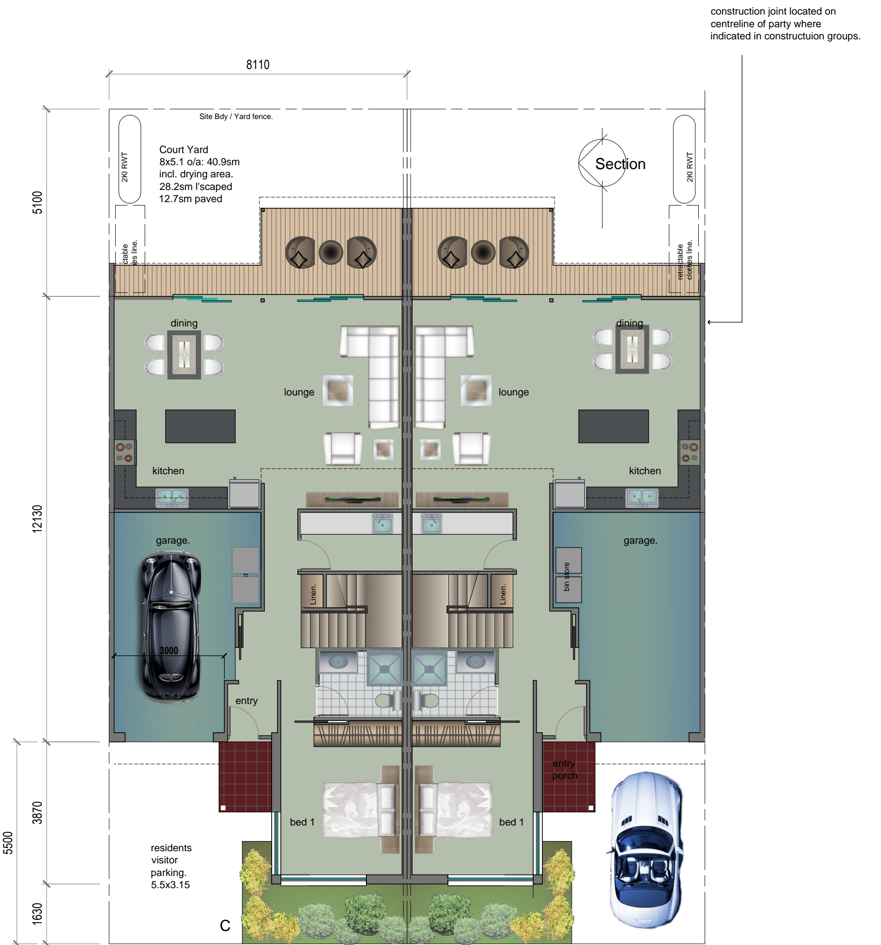
TOWN HOUSE TYPE-C Ground Floor Plan. Floor Area: 89.8 sm.
