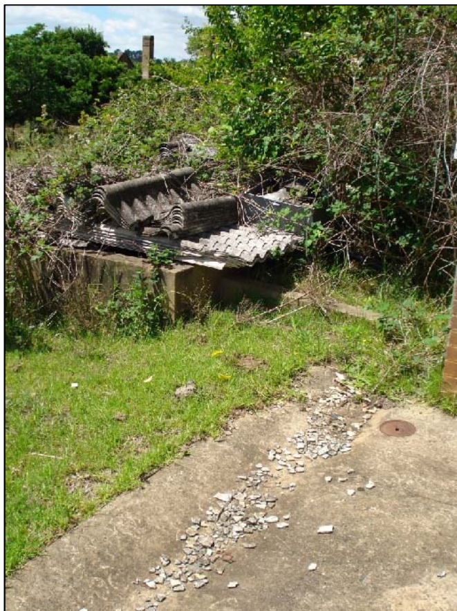
Plate 11: Old abandoned asbestos roofing sheets and numerous fibro fragments located adjacent to old dairy.
