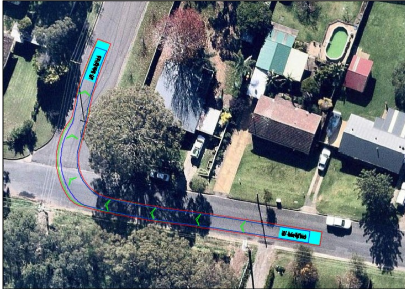
8.8m Medium Rigid Vehicle right turn from Macquariedale Road to Kerr Street Tested @ 10km/h Successful
