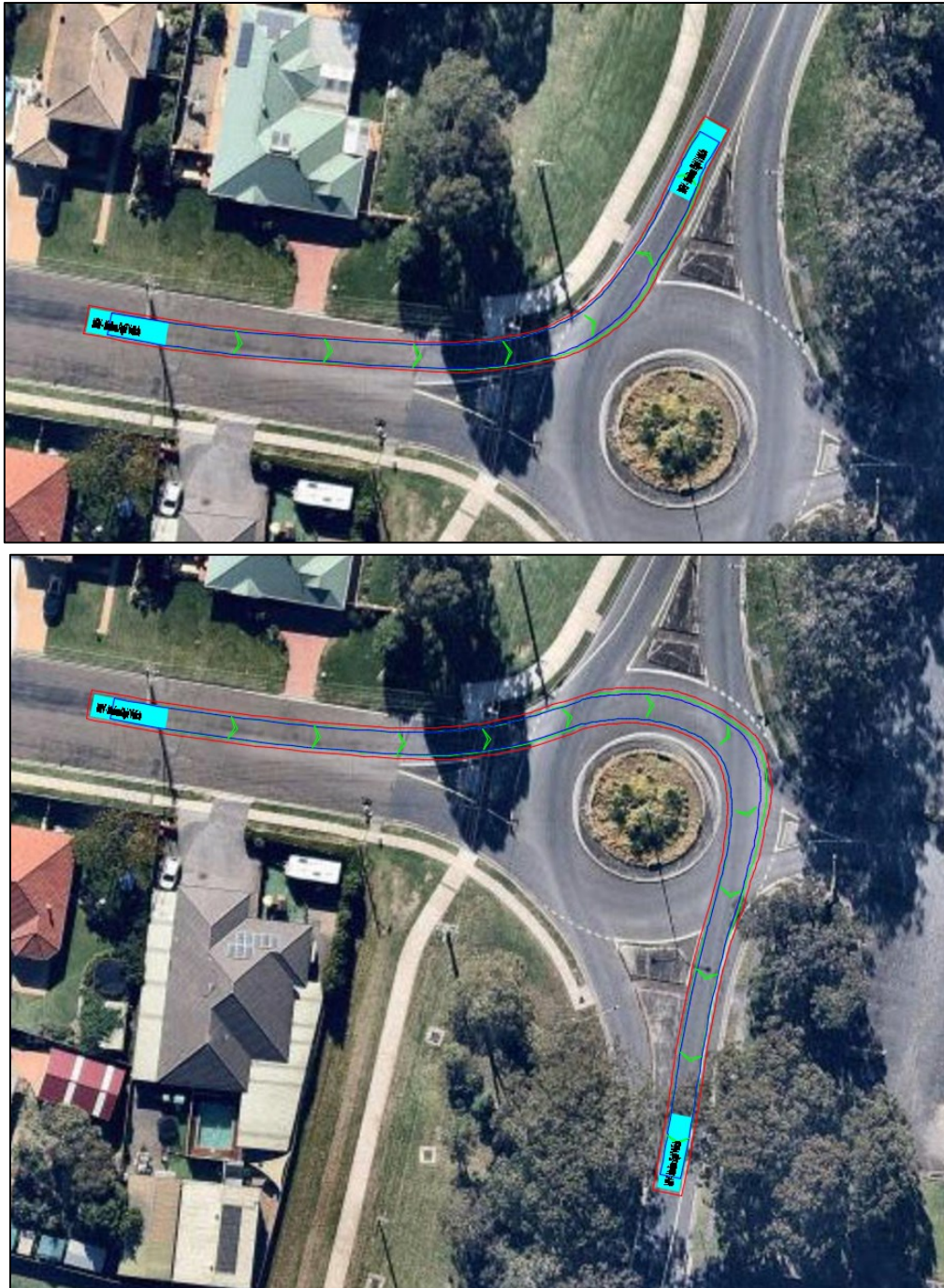
8.8m Medium Rigid Vehicle left / right turn from Rixon Road to Appin Road Tested @ 10km/h Successful
